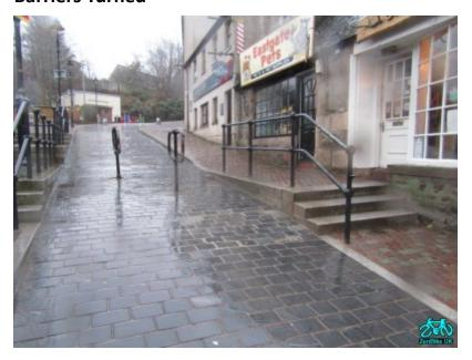
The barriers are normally locked across the route creating a chicane to slow down speeding cyclists. But they can be unlocked and turned for parades etc and fully removed for emergencies. It should be noted that the barriers are across the road. It's footway space that is limited at this pinch point.
